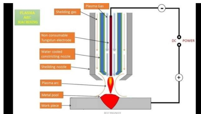
A plasma torch as shown in figure is set up which is also known as the gun or plasmatron, gases such as H<sub>2</sub>, N<sub>2</sub>, O<sub>2</sub>, etc. is passed through an orifice where high frequency arc is setup between the tungsten electrode (cathode) and the copper nozzle (anode) where the electrodes are water cooled.
